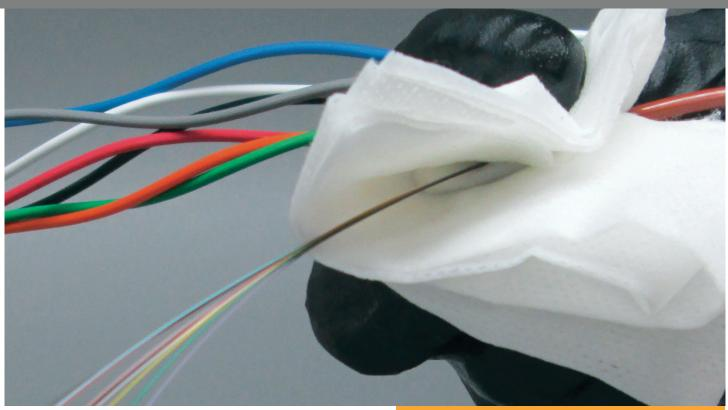
A fast and effective gel remover for loose tube, ribbon, and coaxial cable
