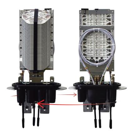
FOCUS CODC2 are the compact version of the ODC2 closures. These closures are externally made of a BASE and a DOME, both available in 2 sizes A and B. The flat rectangular shape allows the installation of the closure inside handholes. The back space of the junction modules fixing STACK can be used as a storage for the uncut cables, containing the optical fibers not involved in the junction.
