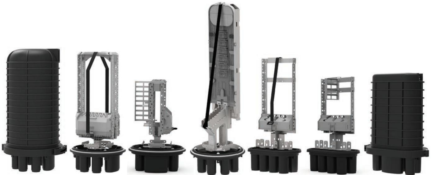
Optotec has a wide range of closures matching every needs in telecommunications networks. They are watertight containers (IP68, IEC 529) able to join and terminate traditional cables and micro-cables with G652 and G657 fibers, used for underground networks, in handholes, manholes and for aerial, wall or pole applications. These types of closures consist of a BASE and a DOME, available in different configurations and customizable according to clients' specific needs.
