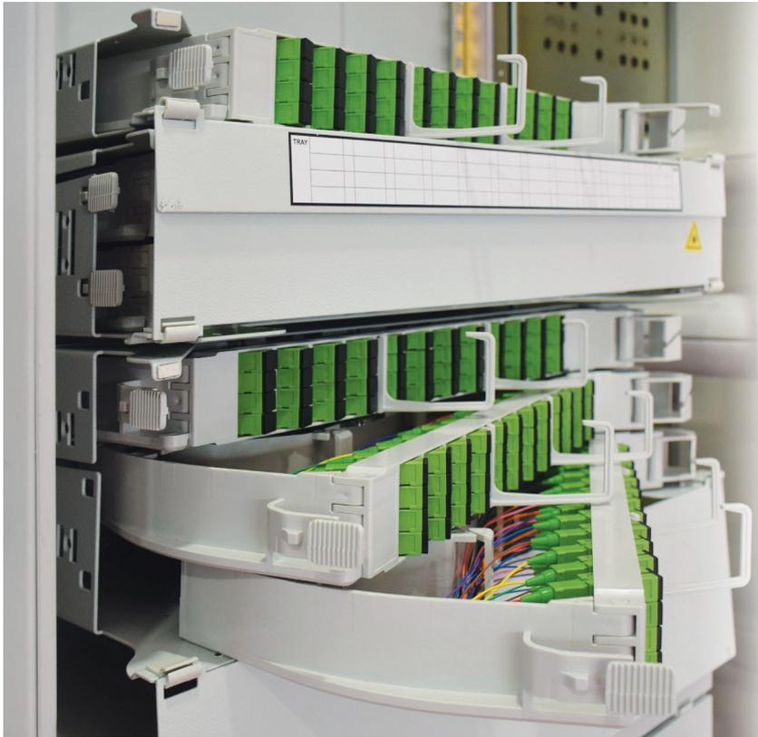
FOCUS-New Pivoting Tray Drawer is suitable for splicing and patching fibre optic cables. The rack (or case) structure of these drawers are 19" in size with a metallic material and a removable front cover. Pivoting trays are mounted inside, right or left opening according to the request.
